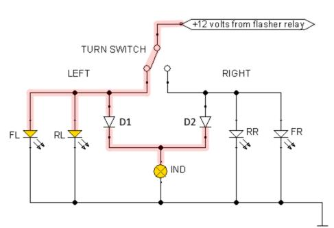
connections with heat shrink tubing. The modification is now complete and your new circuit should look like the diagram on the left.
