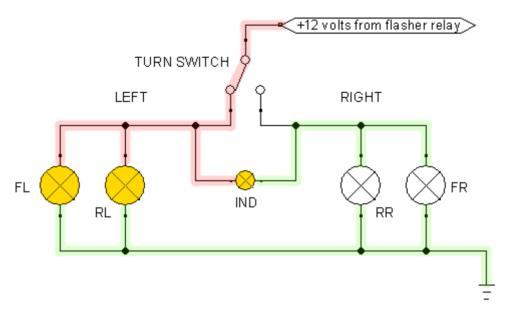
In the illustration you will see that the dash indicator is in parallel with the left side lamps, yet it is in series with the right side lamps, which would beg the question: why does the dash indicator light up without lighting the turn lamps as well? After all, the dash indicator has a wire filament too, so it must be providing power from the turn switch to the unlit lamps. The answer lies in the resistance of the filaments and series connection.
