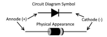
The drawing above shows circuit symbol and actual physical appearance of a diode. The circuit symbol is like an arrow with a bar across. The arrow shows the direction that the diode will let current pass through it, the bar means that if current is fed into the diode from that end, the current will be blocked.
