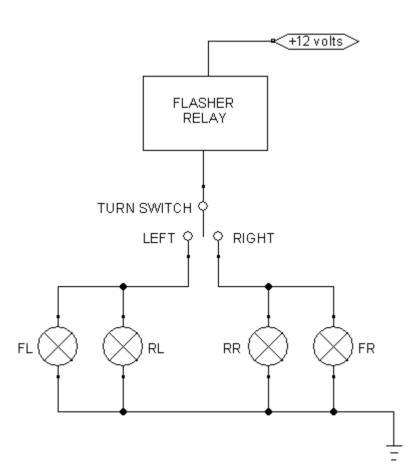
typical turn signal system there are 4 lamps, and these are connected in front/rear pairs to each side. So the Left side has a front lamp and a rear lamp connected together, and the same for the right side. The way that the lamps are connected to each other is called 'in Parallel'. I have marked the lamps in the drawing FL (Front Left), RL (Rear Left).. you get the picture. Now we can look at the individual components.
