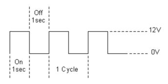
The guidelines in the UK and the USA are that the relay must operate between 60 and 90 cycles per minute, but flasher relays typically operate at 60 cycles per minute. This means that the lamps are lit for one second then extinguished for one second.
